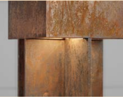
Corten steel or “weathering steel” forms a stable rust-like appearance if exposed to the weather for several years. It was developed in the US during the 20th century and means that due to its chemical composition, this steel exhibits increased resistance to atmospheric corrosion compared to other steels.
